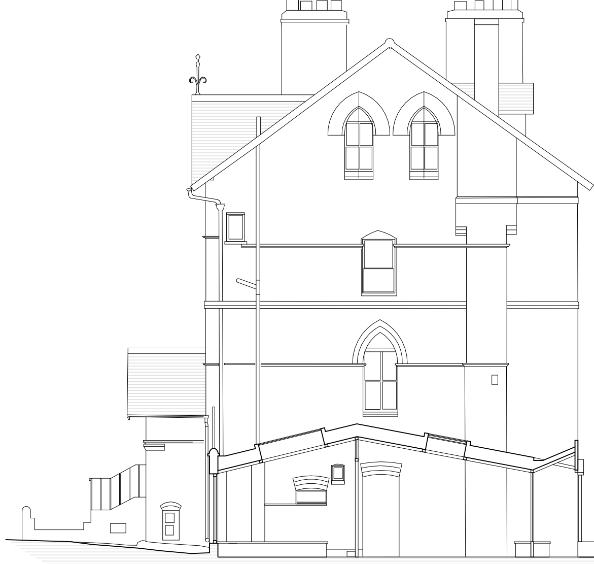
Proposed cross section through new covered entrance, between nos. 6 & 7 Bevington Road
